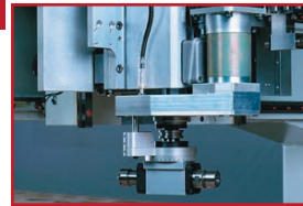
"mcutor" head for 360° - rotation for aggregate
